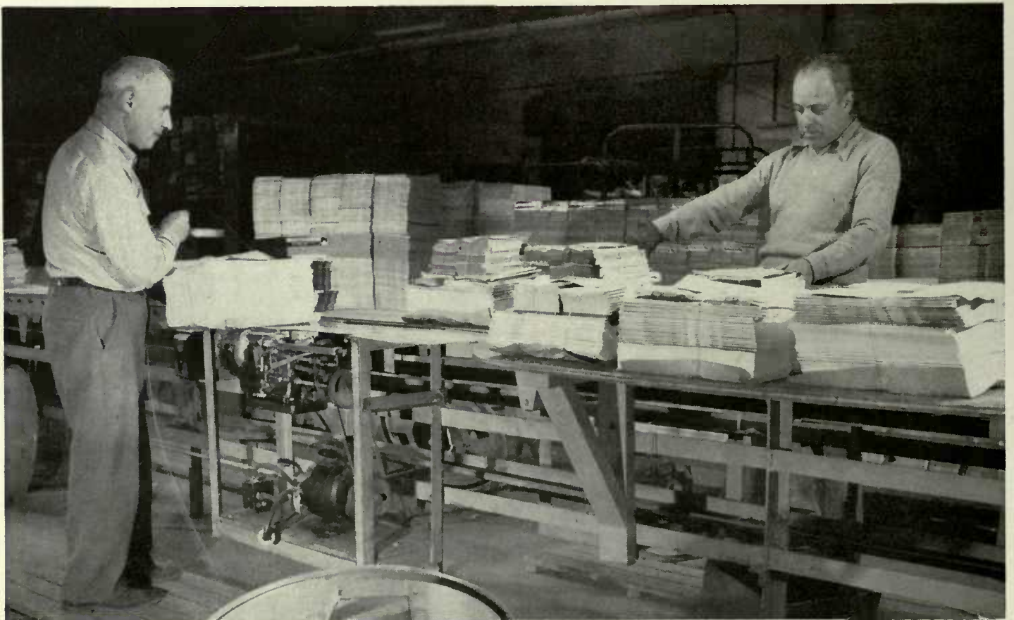
A semi-automatic machine for tying round strapping wire is closely inspected by an experienced workman.
